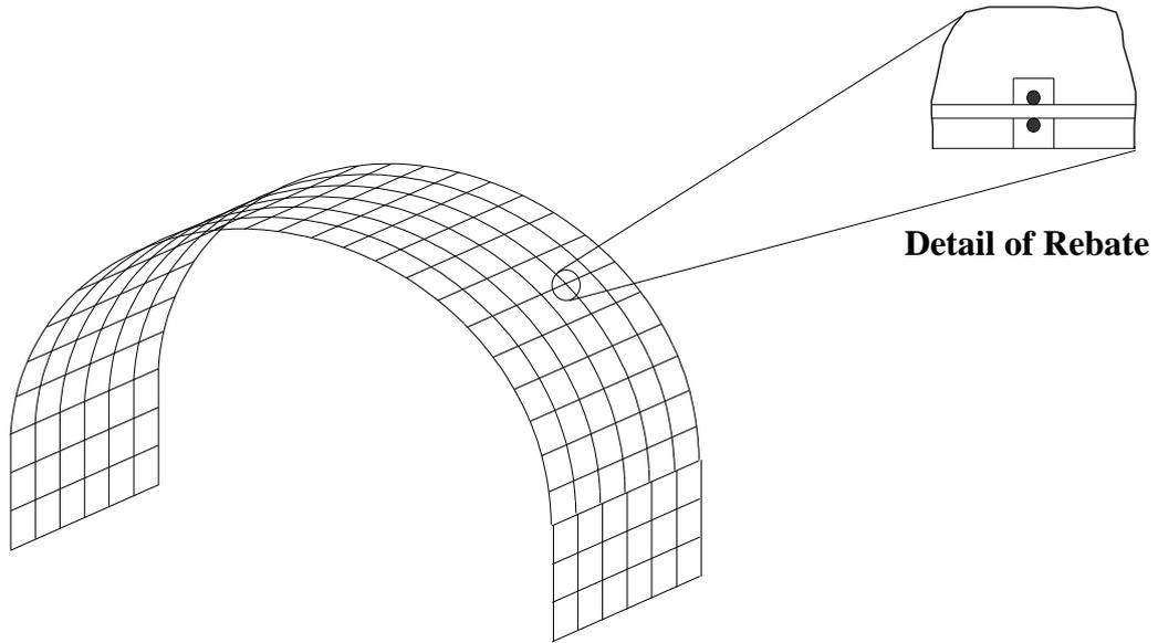
Figure 1 Schematic View of Arch Reinforcement Cage for Barrel only
