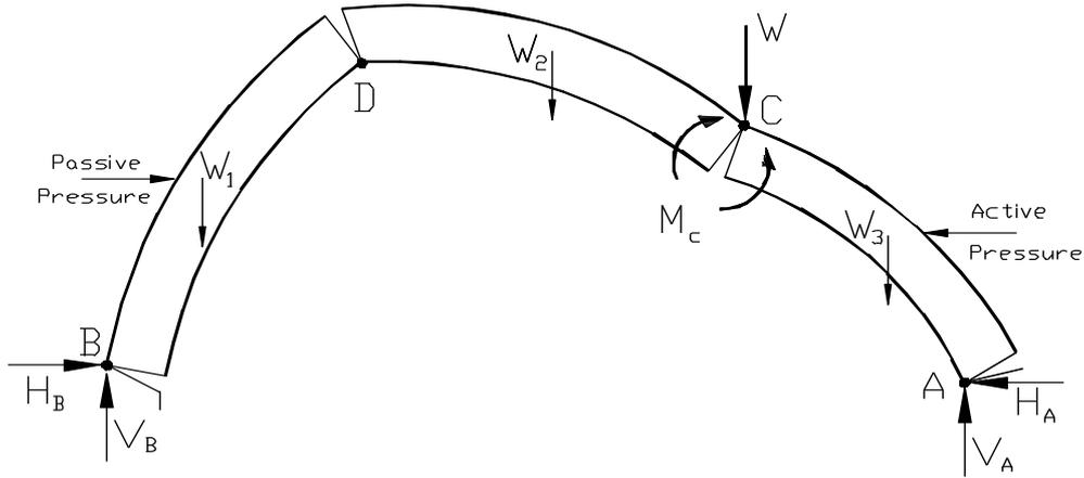
Figure 3 - Forces on Barrel at Mechanism Failure for Reinforced Section
